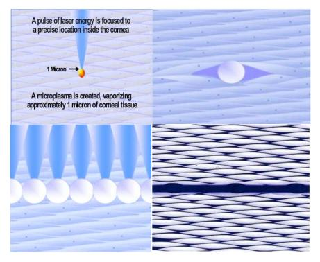
Fig :1. (Clockwise from top left) Focus and application of laser beam; Formation of microplasma bubble; Cavitation bubbles lying close together and Gas bubbles forming a contiguous layer.
